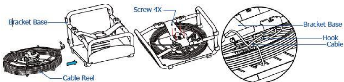
Figure 6. Cable reel in the frame
